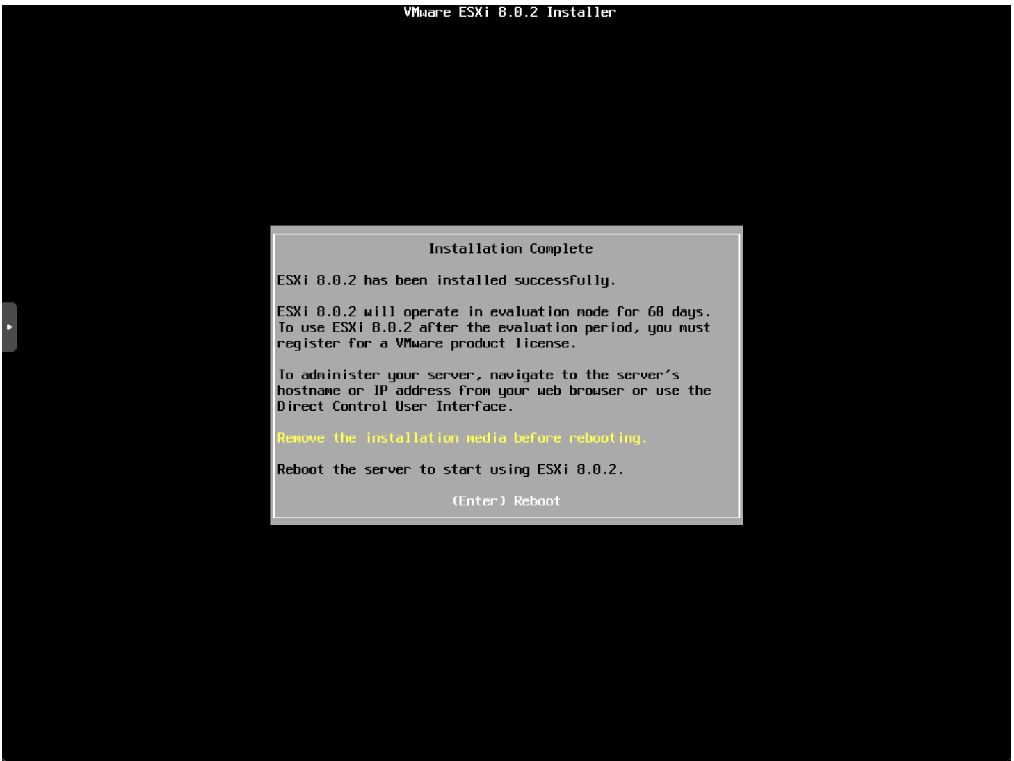
Installation finished remove installation media
